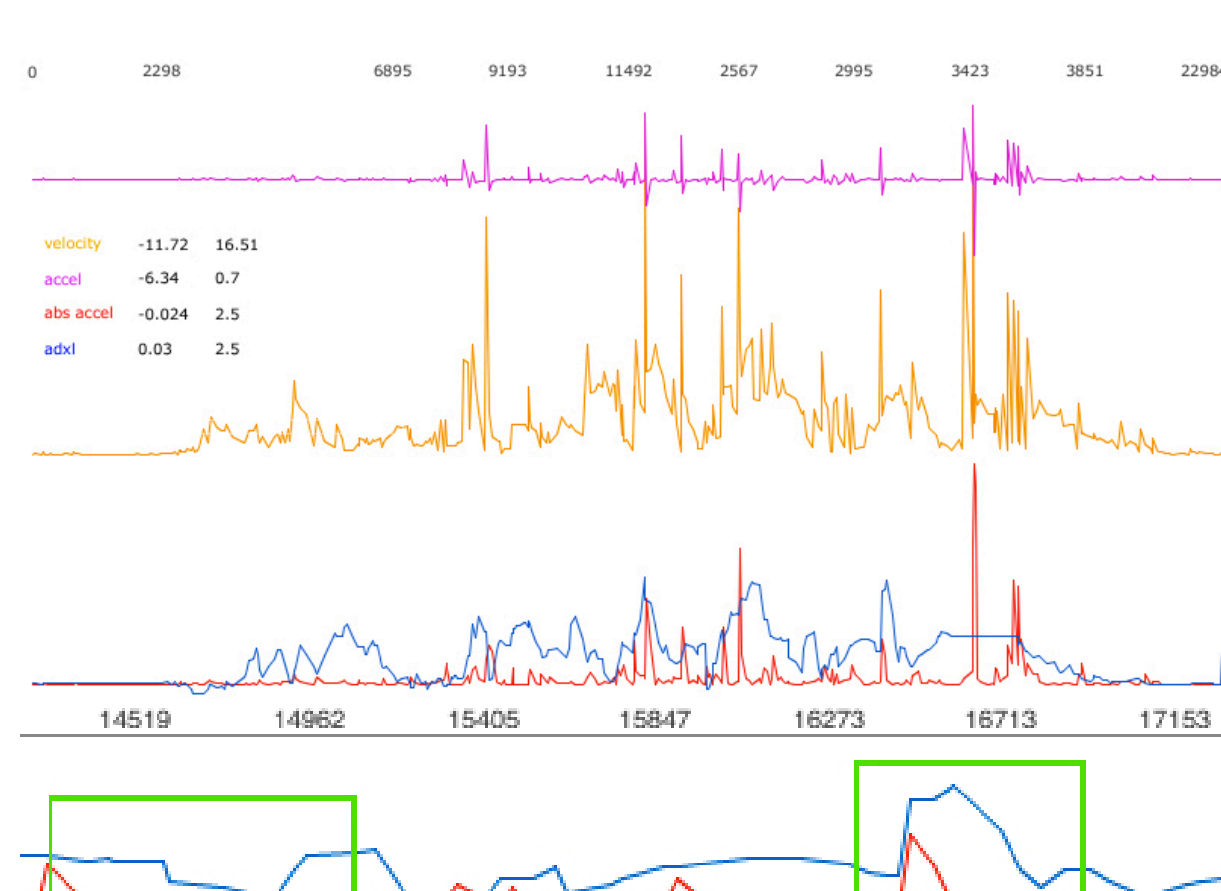
Figure 4. The red line depicts kinematic acceleration extracted from the motion capture; the blue line shows the accelerometer values. Note the overhang in the green boxes, this indicates inertia and co-articulation.
