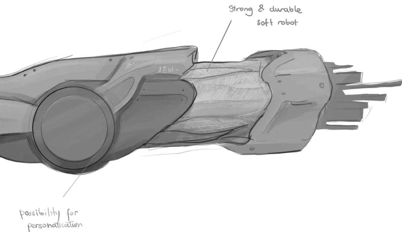
The prosthetic I have developed incorporates both soft robotics and hard robotics to ensure hardware protection. The structural design of the prosthetic embraces various levels of material compliance, each serving specific purposes. For instance, the hand component is intentionally softer, allowing for natural and comfortable interaction with others. This careful integration of soft and hard elements in the prosthetic's structure enhances its overall functionality and usability.
